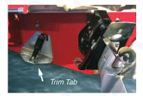
the motor in will lower the bow. Trim tabs adjust the boat's list (right and left balance).
