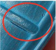
Check the primer bulb for cracks!
