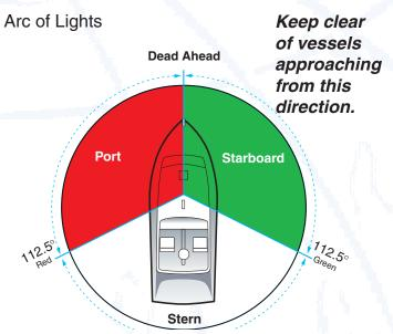
**Masthead light** means a white light placed over the fore and aft centerline of the vessel showing an unbroken light over an arc of the horizon of 225 degrees and so fixed as to show the light from right ahead to 22.5 degrees abaft the beam on either side of the vessel
