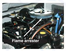
Ignition protected components prevent electrical sparks from igniting fuel fumes and vapors emitted from gasoline, engines, generators and fuel burning appliances.
