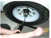
Don't forget to grease the bearings!
