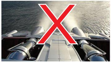
A muffler system in good working order must be used at all times when the vessel is operated within 5 nautical miles (9.26 km) of shore.
