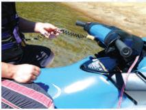
Attach the safety lanyard. machine c it circling around you and perhaps running over you.
