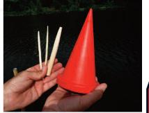
Tapered wooden plugs or this orange sponge like device can be used to slow or stop a leak!
